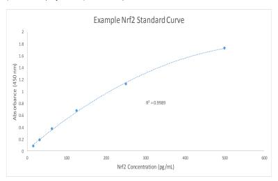
Note: Inclusion of the high standard is optional. When samples are found to be in the lower portion of the curve, omission of the high standard can sometimes provide a more accurate curve fit and thus better results.
